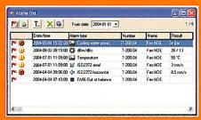
Alarm lists are generated on the basis of automatically applied evaluation rules that can be modified by customer-defined thresholds. You also can program alarm-delay conditions, log all alarm messages on a printer and connect any or all measuring channels to the main alarm relay.
