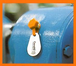
Contact-free ID tags store the measuring point data along with the latest measuring results. The transfer of data and measuring results occurs via radio transponder between the logger instrument and the ID tag.
