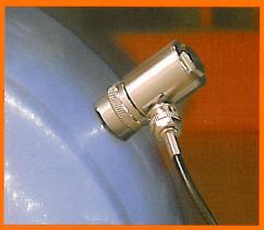
Special transducers are available for measuring points that are inaccessible during normal operation. The transducers are permanently installed and connected via cables to measuring terminals
