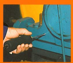
Speed data is necessary for condition evaluation and monitoring machine temperature often supplies valuable information. The machine tester uses temperature probes for solids and liquids. Speed can be measured by contact or noncontact means.
