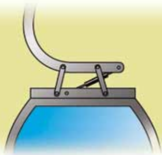
Swinging movements cushioned by hydraulic dampers
